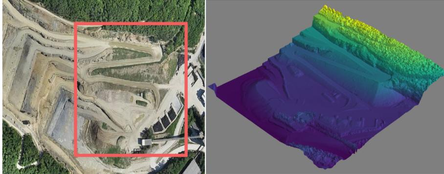
**Fig. 7.** Heightmap extracted from Sensefly’s mining quarry dataset [19]. Reference top-view image and perspective view of the elevation map from the extracted red region are shown at left and right respectively.
