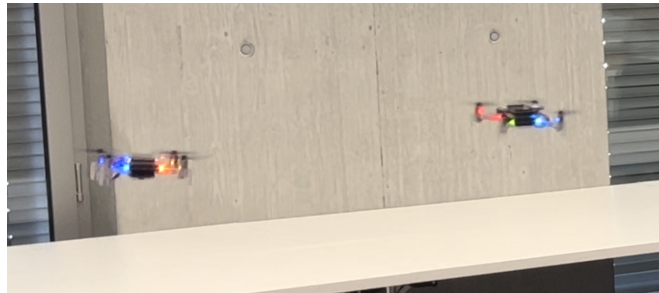
Fig. 1. Our in-field system: one nano-drone visually estimates the relative pose of the other.
