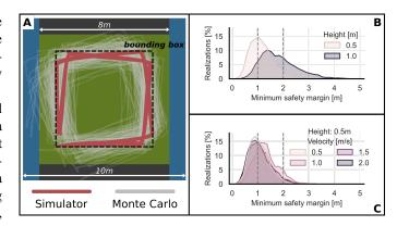
Fig. 3. A) 1024 simulated Monte Carlo trajectory realizations B) minimum safety margin w.r.t. height, C) minimum safety margin w.r.t speed, having fixed the height to 0.5 m.
