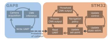
Fig. 5. The drone's state machines mapped on the MCUs available aboard.
