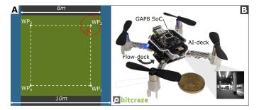
Fig. 2. A) the  $10 \times 10$  m competition arena. B) the robotic platform.
