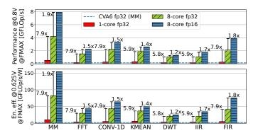
Fig. 14: Performance and en. eff. delivered by the cluster on general-purpose DSP benchmarks.
