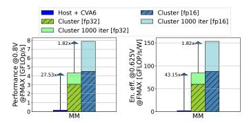
Fig. 12: Offload performance breakout on an FP MM.
