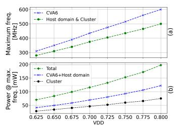
Fig. 10: Maximum frequency and power envelope varying VDD.
