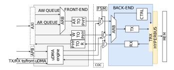
Fig. 4: HyperRAM memory controller architecture.
