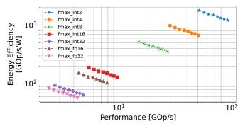
Fig. 11: Pulp cluster energy efficiency on dense matrix multiplication. 1 MAC = 2 Op.
