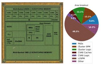
Fig. 8: Die micrograph (3mm x 3mm) and area breakout.
