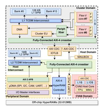
Fig. 1: Shaheen architecture block diagram.
