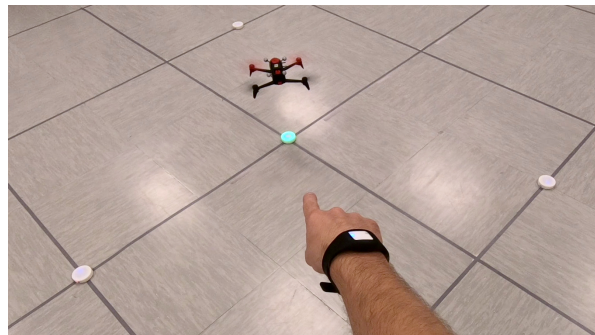
Fig. 1. First person view of the operator equipped with a wrist-mounted IMU interacting with a quadrotor.
